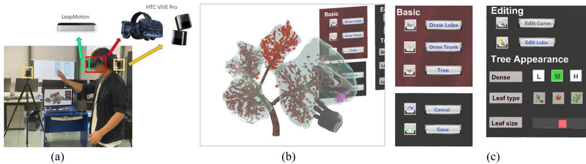
Figure 2: Our mid-air sketching based tree modeling system. (a) Hardware setup: an HTC VIVE VR glass with Leap motion. (b) The workspace from a user’s perspective. The 3D movements of hands are directly captured by Leap motion. (c) The control panels that allow the user to switch the modeling stages and manipulate the tree appearance.
